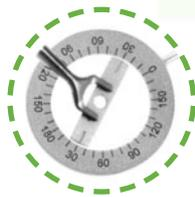
A simple method of marking the steep meridian is with the Bores axis marker aligned in the Mendez degree gauge.
